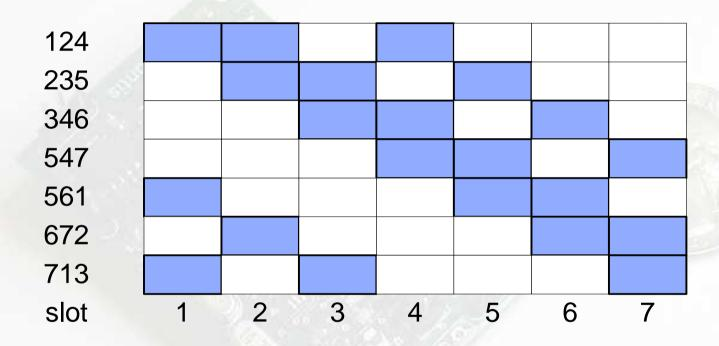
An example of asynchronous schedule based on a symmetric (7,3,1)-design of the wakeup schedule function.
