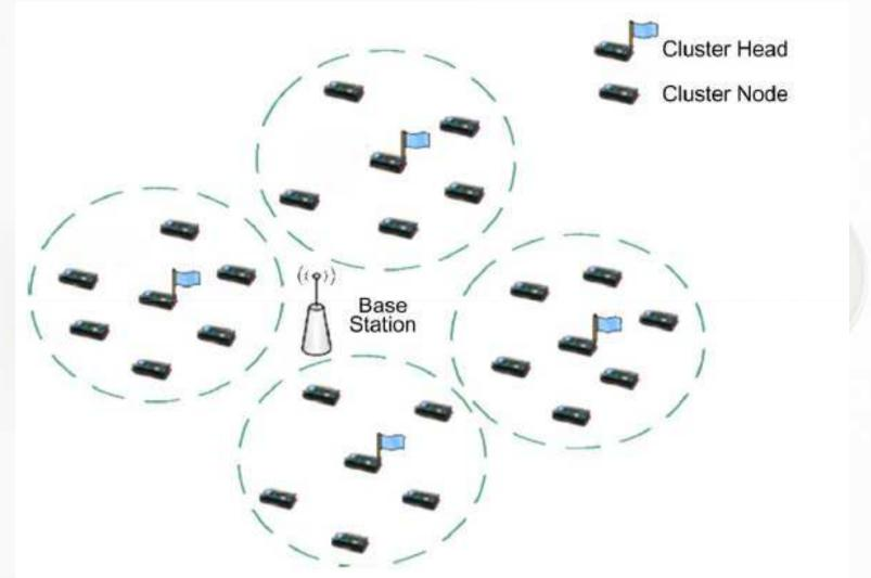
Cluster Heads also use a TDMA approach for sending data received from Cluster Nodes to the Base Station
